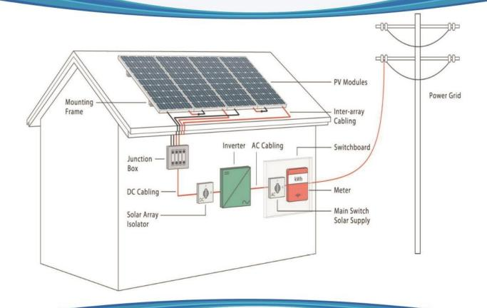
The PV system is interfaced with the state power utility grid. The solar power runs the load to the extent possible during day time. If there is excess energy generated, the same is exported to the power utility grid. If there is a deficit in energy generation, the differential Power/Energy is drawn from the grid. A bi-directional meter will be installed to record the net energy.
