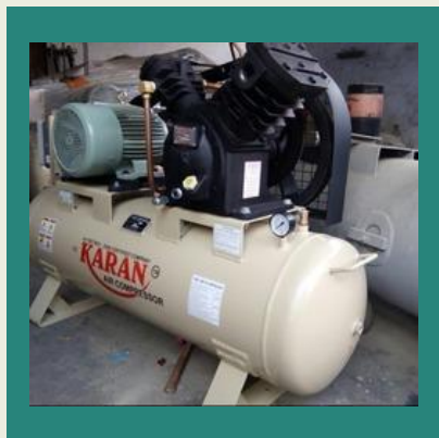
Two Stage Compressor
