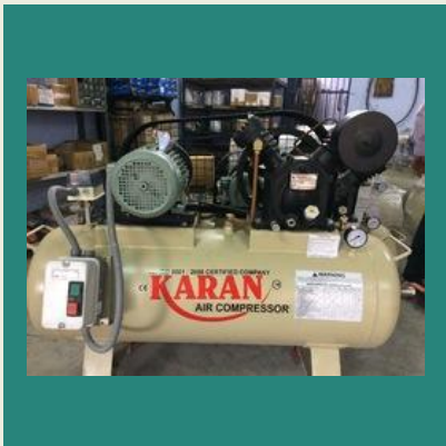
Air Cooled Compressor
