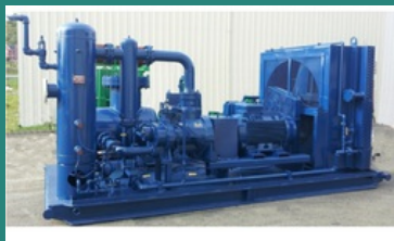
Motor Driven Compressor
